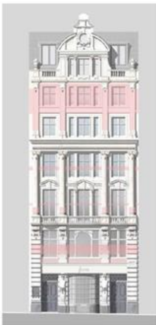
Consented 4-6 Glasshouse Street Elevation showing new Portland stone inserts above ground floor
